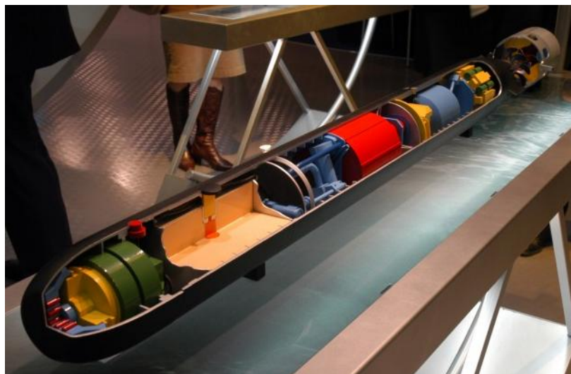
A cut-away model of the WASS SpA Black Shark torpedo, on display at Euronaval, France
