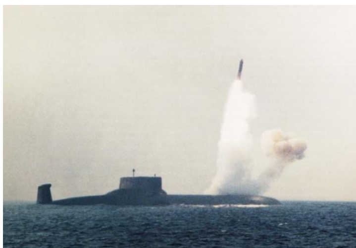
A Bulava SS-NX-30 ballistic missile being test launched from the Typhoon-class submarine Dmitriy Donskoy
